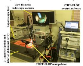
Fig. 1 Test set-up
