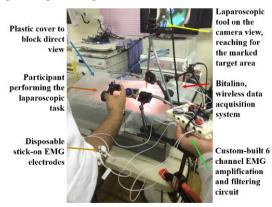
Fig. 2 EMG acquisition during the laparoscopic test
