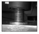
Fig. 11. Misalignment error. The robot places the nut on a faulty angle which causes the nut to be stuck on the bolt as soon as tightening process is started.
