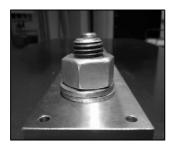
Fig. 12. The 'two washers' error scenario. The  $2^{nd}$  washer will cause an error detection within *stage 3* or 4, since the desired angular position of the nut will not be reached.
