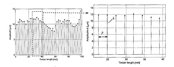
Fig 8: Surface profile recreation by using spindle vibrations
