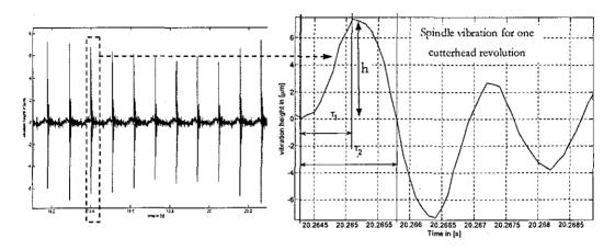
Fig 6: Spindle vibrations during the machining process
