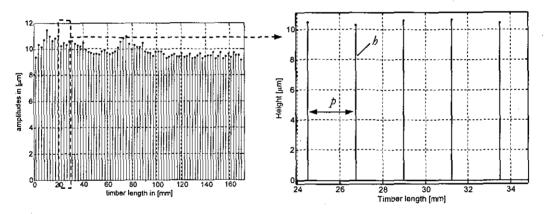
Fig. 5 Re-created surface profile by using spindle speed
