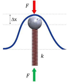
The distance between the sphere and the camera varies with the interaction force.
