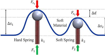
$$K_{S} = \frac{F_{1} - F_{2}}{\Delta s_{1} - \Delta s_{2}} = \frac{K_{1} \Delta x_{1} - K_{2} \Delta x_{2}}{\Delta d}$$
