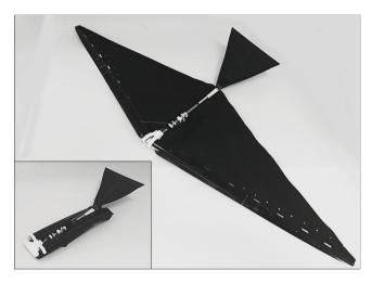
Figure 3. Deployable glider module for multimodal robots
