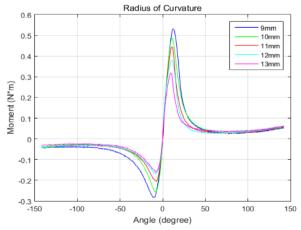
Figure 2. Experimental result of the folding angle v.s. joint torque of the curved compliant facet origami structure
