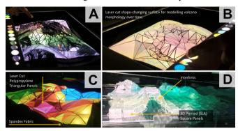
Figure 2: Semi-Solid laser cut surface for modeling a shape-changing volcano morphology (A-B). Breakdown of laser cut semi-solid surface structure (C). A 3D printed surface used to show oceanography wave simulations (DC).
