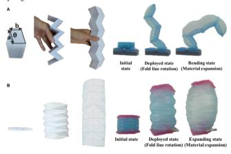
Figure 2. (A) Miura-ori polyhedron inspired soft robotic origami structure. (B) Yoshimura patterned cylinder inspired soft robotic origami structure. Both structures has sequencial motions: origami-like motion and soft robotic motion
