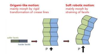
Figure 1. Principle of soft robotic origami structure. The structure deploys by origami-like motion
