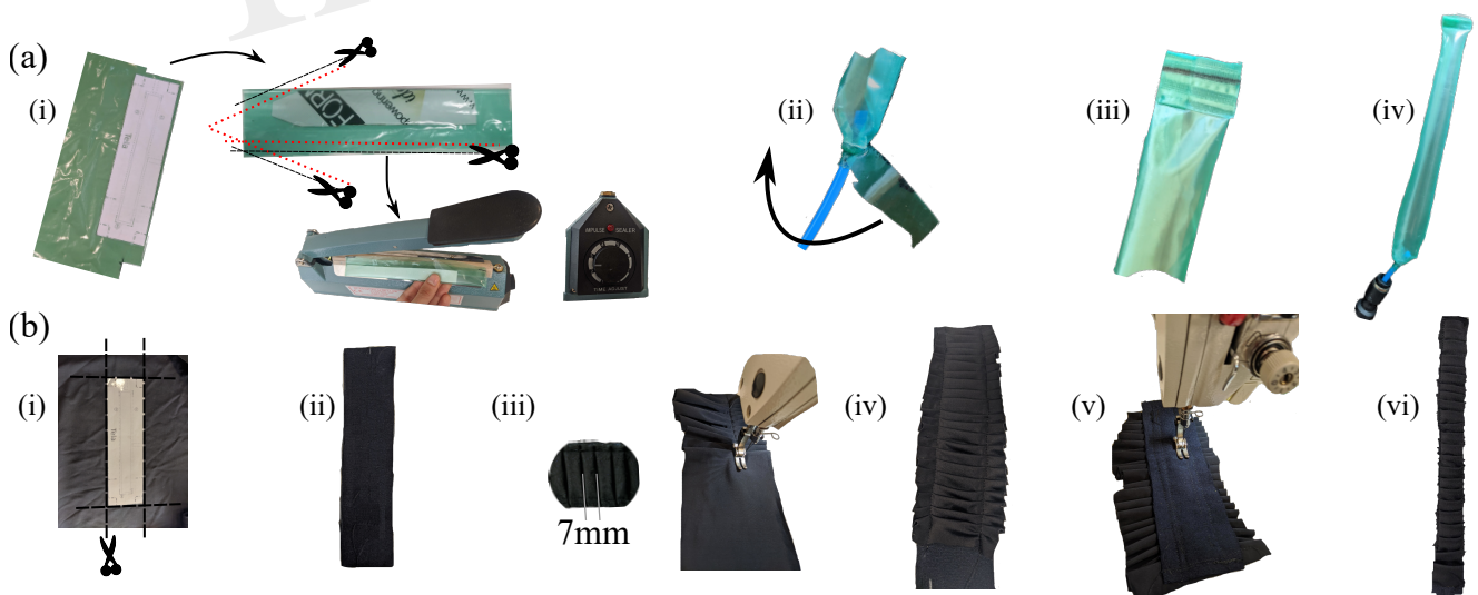
Figure 3. The construction process of a textile actuator with pleats. (a) Construction of the internal balloon keeps the air in the actuator; (a-i) Cutting the plastic and sealing with the impulse sealer machine. (a-ii) Placement of the plastic tube for inflation. At this point, plastic reinforcements are added to prevent leakage at the joint. (a-iii) Sealing the end of the actuator several times to avoid leaks. (a-iv) The pressurised balloon is shown. (b) Construction of the textile pocket with pleats; (b-i and b-ii) Cutting the rigid and elastic fabric. (b-iii) Joining the elastic fabric over the rigid one while making the pleats. (b-iv) Pocket with pleats sewn on both sides. (b-v) Definition of the actuator width through a line made with the sewing machine. (b-vi) Cutting out excess fabric from the pocket.
