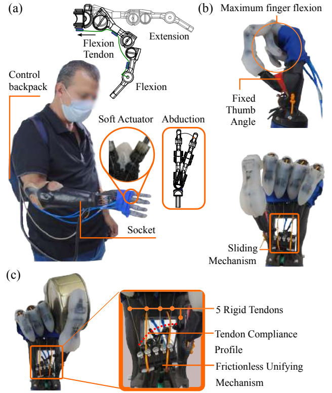
Fig. 1. PrHand V2 underactuated Soft-Robotic prosthetic hand. a) Amputee user adaptation and illustration of finger flexion and extension (a tendon-driven compliant mechanism) and abduction degree of freedom driven by a soft silicone actuator. b) PrHand V2 prosthesis enhancements. c) Compliant grip example showing how a compliant profile is generated in the elastic tendons, adapting to the shape of the object gripped without needing prior control.
