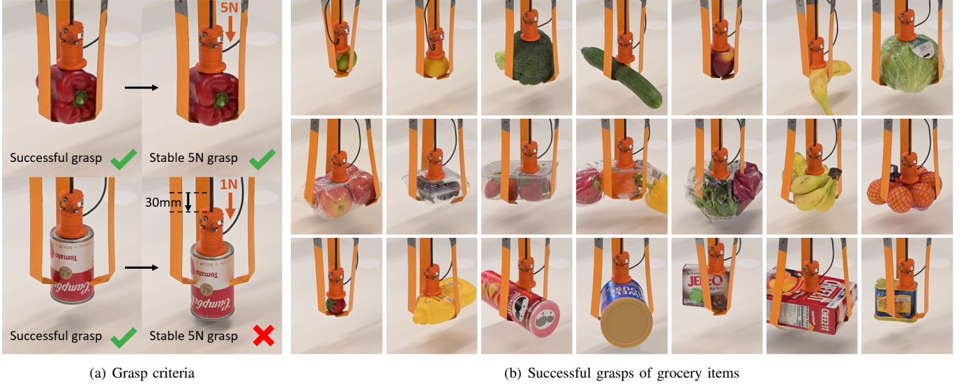
Fig. 6. Grasps achieved using our PPO policy; a) Illustrating the two criteria used to evaluate grasps: a successful grasp requires a lifted object and safe finger and palm forces (1 – 4N), whereas a stable 5N grasp requires tolerance to a 5N vertical disturbance from the palm, which pushes downwards up to 30mm whilst measuring whether the required force exceeds 5N; b) Grocery item grasps, real in the top two rows and YCB [46] in the bottom row.
