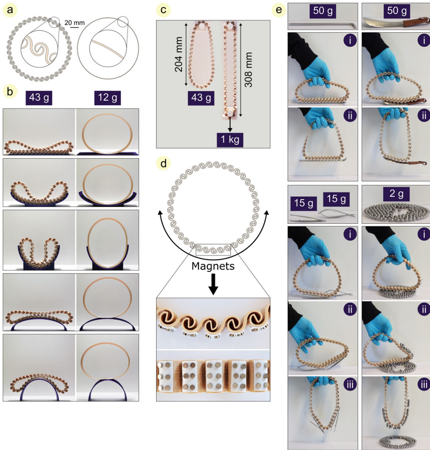
Fig. 9 Freeform passive gripper. a Models of double-spiral and circular loops, illustrating their structural differences. b Interaction of the double-spiral and circular loops with flat, concave, and convex surfaces, demonstrating deformation under their own weight. c Elongation of the double-spiral loop caused by its own weight and an additional 1 kg load. d Small disc magnets attached to the lower half of the double-spiral loop using double-sided tape, with close-up views from the top and side perspectives. e The spiral-based magnetic gripper used to lift a 50 g Allen wrench, a 50 g shoehorn, two 15 g tweezers, and 2 g steel beads. Reproduced from [17], licensed under CC-BY 4.0
