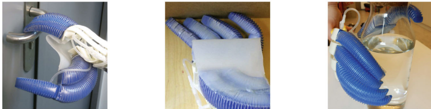
Fig. 3 Examples of bad morphological computation. Left: soft fingers yield while pulling on a heavy door handle. Middle: fingers buckle while sliding along a wall. Right: fingers buckle while lifting a heavy bottle (photos reprinted from [24] with permission, © 2017 IEEE)
