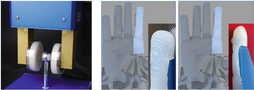
Fig. 13 Supplementing a conventional gripper by using thermosensitive hybrid materials (left) as well as shape adaption and morphology changes (contact area) to generate new morphological features for gripping of objects (right)
