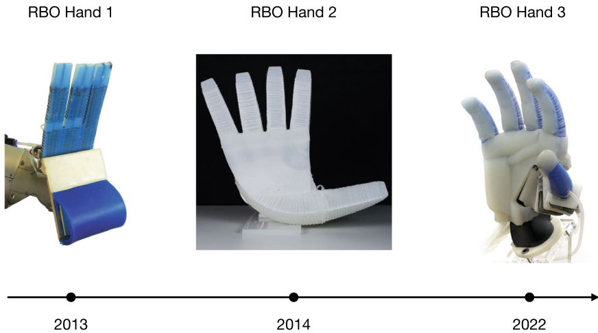
Fig. 1 Three generations of RBO Hands: RBO Hand 1 (photo reprinted from [6] with permission, © 2013 IEEE), RBO Hand 2 (photo reprinted from [7] with permission of the authors), and RBO Hand 3 (photo reprinted from [8], licensed under CC BY 4.0). Anthropomorphism increased over time, driven by improvements in thumb dexterity
